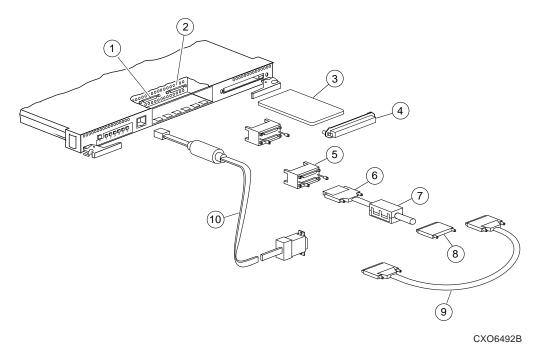
Figure 1–4. Parts Used in Configuring the HSZ80 Array Controller
